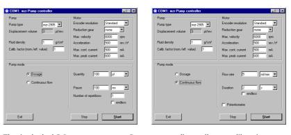
The included PC program »mzr-Pump controller« allows calibration, programming of volumes, flow rates, pause times, cycle numbers and dosage time and setting of drive parameters. Displacement volume and flow values can be selected for standard mzr-pumps. Simple dispensing tasks can be programmed.
